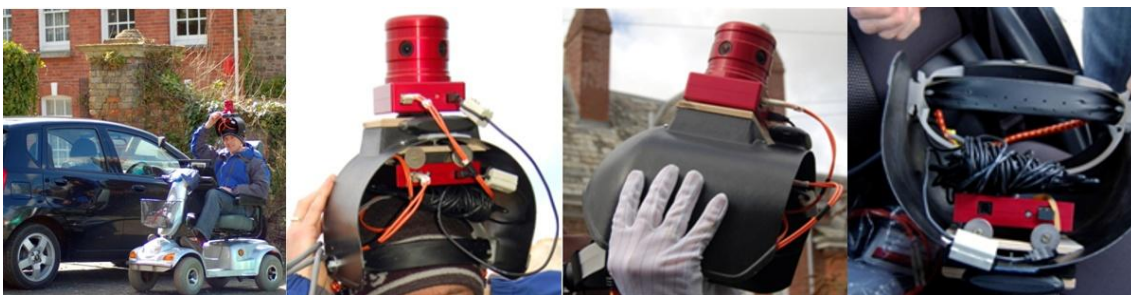
Figure 69 The application of a mobility scooter and a welding helmet in the first approach of creating a mobile camera system. Images by Karol Kwiatek.
