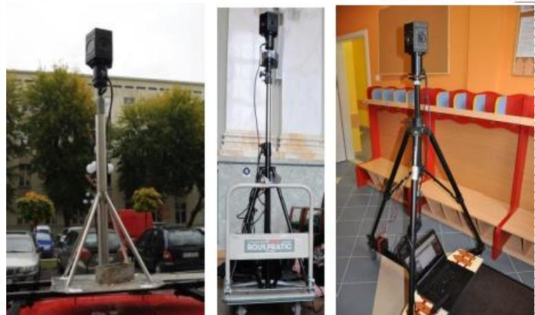
**Immersive camera** - a digital camera that captures 360° video that is recorded from frame cameras with individual projection centers
